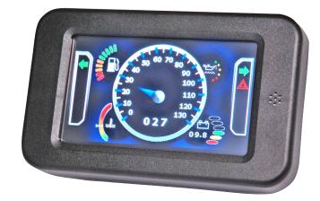
The 550MDI (Media Display Interface) is a CAN based 4.3" 262K color 480 x 272 TFT High Brightness LCD with touchscreen. The 550MDI supports dual independent CAN transceivers and a LIN transceiver for providing a gateway between multiple in-vehicle networks.
