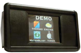
The 591CANDI (CAN Display Interface) is a CAN based 2.4" 262k color 320 x 240 TFT LCD with resistive touch screen. The 591CANDI supports multiple CAN protocols including J1939 and CANopen. The resistive touch screen allows usage in harsh environments or with heavy gloves.
