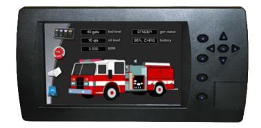
The 700MDI (Media Display Interface) is a CAN based 7.0" 262K color 800 x 480 TFT High Brightness LCD with touch-screen. The 700MDI supports dual independent CAN transceivers for providing a gateway between multiple in-vehicle networks. Screens are designed using an intuitive GUI builder (CANcreate) capable of implementing dynamic customer interfaces.
