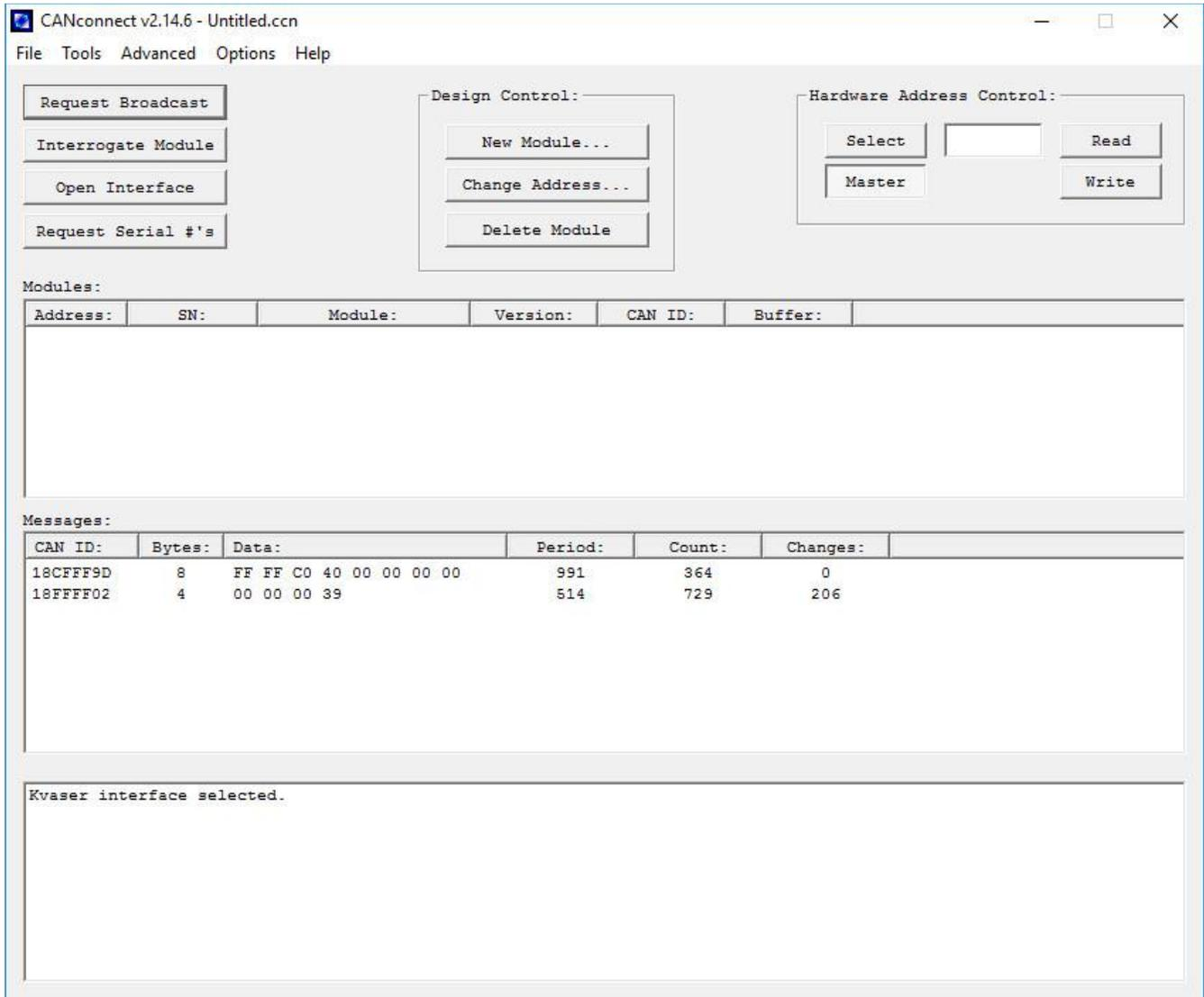
This is the main CANconnect window. Through it, all USB connected modules may be monitored and edited through separate interfaces. The various components of the workspace are detailed in this chapter.
