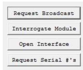
**Request Broadcast** - Locate any attached modules. The modules will show up in the Modules box and corresponding messages in the Message box.
